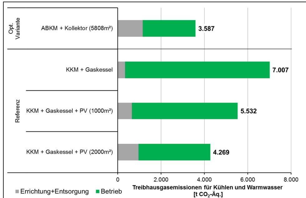
**Figure 12: Case study „Absorption chiller H<sub>2</sub>O-LiBr, refrigeration capacity 1470 kW“: greenhouse gas emissions of the solar thermal optimized variant “Absorption chiller + collector (5808m<sup>2</sup>)” and the reference systems for cooling and hot water at a life cycle of 20 years**
