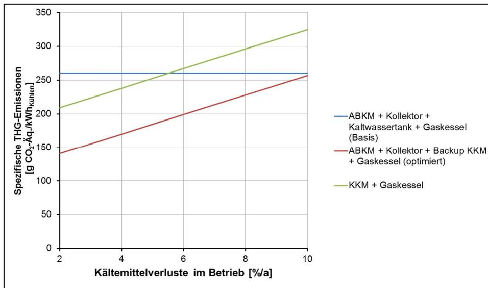
**Figure 13: Greenhouse gas emissions of solar thermal variant and the reference system "compression chiller + gas boiler" with a refrigerant emission factor of 10% during the operational phase (lifetime 20 years)**
